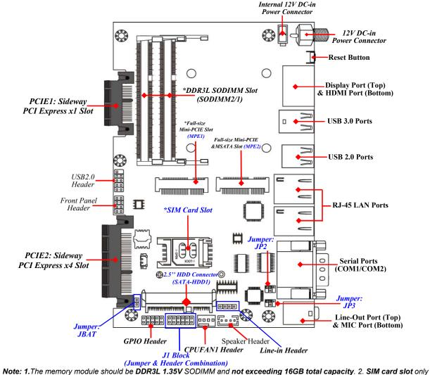
work when compatible SIM card installed & 3G LAN card installed in MPE1 Mini-PCIE slot.
