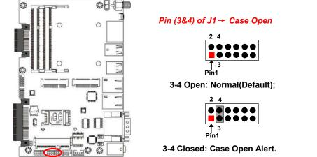
**Pin (3&4) Closed**: When Case open function pin short to GND, the Case open function was detected. When Used, needs to enter BIOS and enable 'Case Open Detect' function. In this case if your case is removed, next time when you restart your computer, a message will be displayed on screen to inform you of this.
